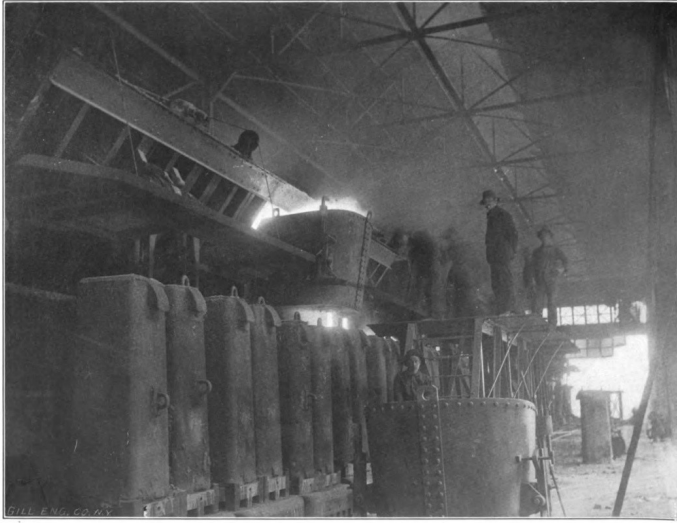
Pouring a Heat from a 50-Ton Open-hearth Furnace, using Fore-hearth, Ensley Steel Works
